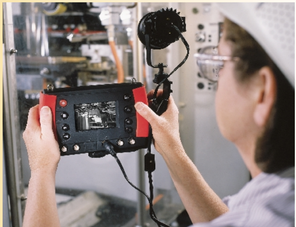
Hand-held system records images at up to 4 sec of recording time, for a total of 4,096 frames. Plays recorded frames on a built-in LCD screen, above. Big G uses it to monitor cereal packing lines and others.
